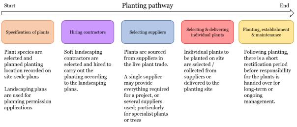
*Figure 1 - Simplified planting pathway for large-scale landscaping projects. In reality, projects are more complicated and less linear than shown here*
